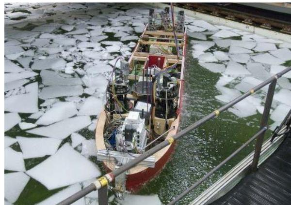
Figure 16: Stena Icemax model during stationkeeping tests in managed ice conditions (19)
