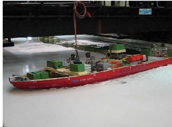
Figure 18: Model tests for ice breaking in transverse direction (24)
